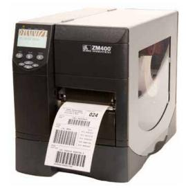
The ZM400 and ZM600 printers bring added flexibility to the popular Z Series platform, offering an easier to operate form, increased connectivity, RFID readiness as standard and an impressive number of available options. They come standard with features that provide unsurpassed easy to use operation and user selectable adjustments such as an adjustable black mark / label edge sensor.
